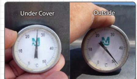
Form temp. inside Rollcov-R: 79°F/26°C Form temp. outside Rollcov-R: 120°F/49°C
